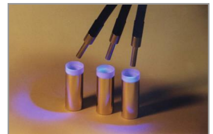
Trifurcated wand curing metal-to-plastic assembly
