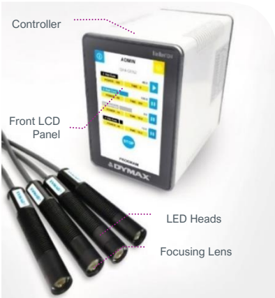
Figure 1. Main Components of a BlueWave QX4 V2.0
