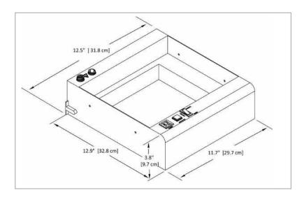
Operation of the shutter is easy and precise control of exposure times can be achieved with by using the unit's two modes of operation: Timed and Manual. In timed mode, the shutter opens by pressing a button on the front switch or by activating the remote switch (i.e. foot switch), and remains open for a user-specified period of time. In the manual mode, pressing the button on the front panel or remote switch (i.e. foot switch) opens the shutter and releasing the button closes the shutter.
