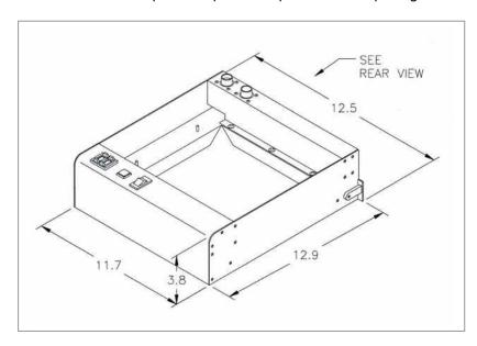
Dymax flood lamps require a few minutes to warm up after ignition. Turning the lamp off and on negatively affects the lifetime of the bulb. With a Dymax shutter installed, the flood lamp may stay on continuously. Objects may be loaded and unloaded from beneath the shutter when it is shut without exposing operators to ultraviolet light. In addition, precise control of exposure times can be achieved.
